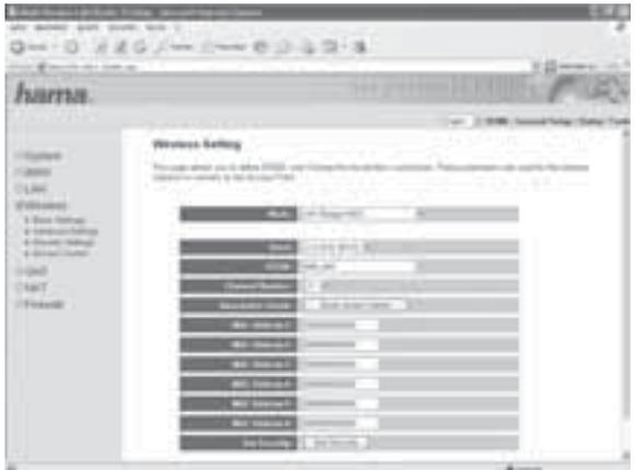
**Channel Number** allows you to select the channel in which the data is to be transferred. 13 channels are available. Enter the addresses of the access points to which the bridge connection is to be made in **MAC address 1 to MAC address 6**. To set the encryption for your wireless network, click the **Set Security** button.
