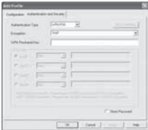
To use **WPA2 encryption**, select **WPA2-PSK** under Authentication type and **AES** under Encryption.
