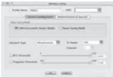
This device allows you to set up two different network types. Select **Infrastructure** under Network type, if you want to connect to a router or access point. The settings for **TX Power**, **RTS Threshold** and **Fragment Threshold** can be left at the default settings.
