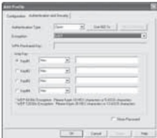
You can now store four codes in the lower section of the window. The selected code is always used. 64 bit or 128 bit encryption is supported. 128 bit encryption is more secure. First select whether you want to use **Hex** (allows characters from 0-9 and a-f to be used) or **ASCII** characters (You can use any characters). The setting and the selection of either 64 or 128 bit encryption determines the length of the code to be entered.
