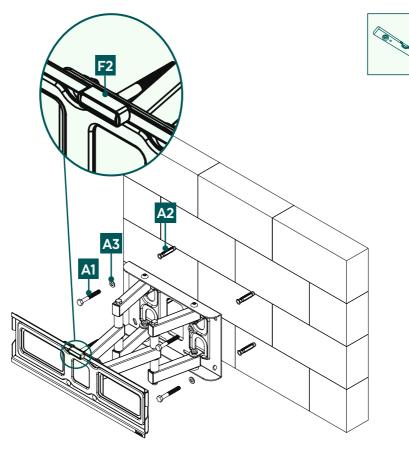
• Attach the wall bracket to the wall as shown above using the enclosed mounting material ([A2] plug, [A3] M8 washer, [A1] 8x60 mm screw and the [F2] spirit level).
